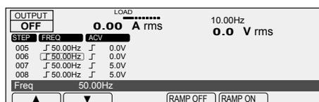
Press ▼ to move the border to the frequency of step 007. Then, use the rotary knob to specify 80.0 Hz. Likewise, set steps 8 and 9 to 40 Hz. Then, press ▼ to move the frequency of step 010.
