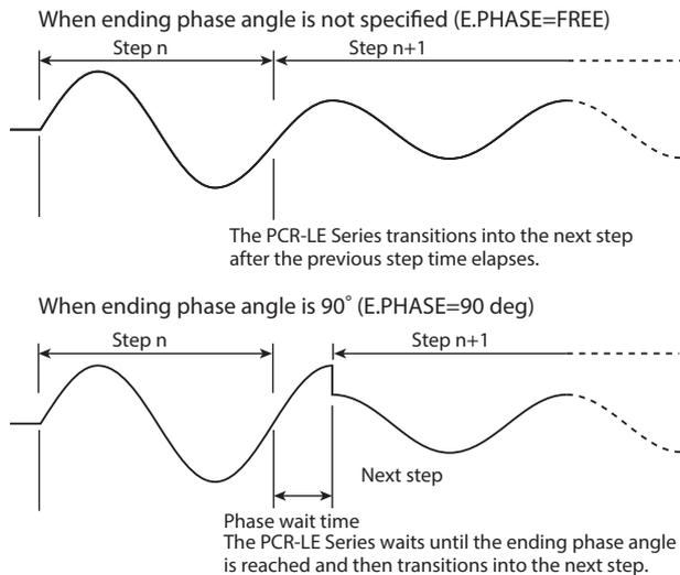
You can output the same waveform regardless of whether you set the starting phase angle or the ending phase angle.
