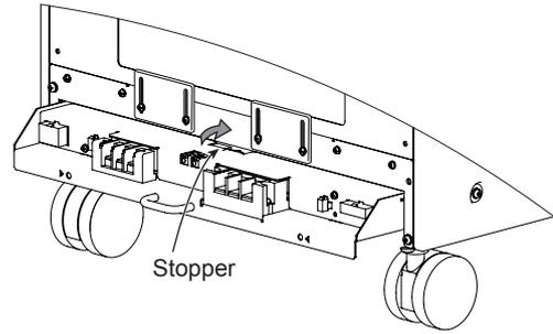
**5** Connect the wires and cables to the terminal block and connectors as necessary.
