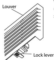
With your fingers, push up on the lock lever under the detachment mark (1), and slide the louver to the right (2).
