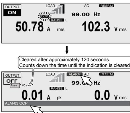
If the internal semiconductor protection is activated repeatedly, the PCR-LE Series may malfunction.
