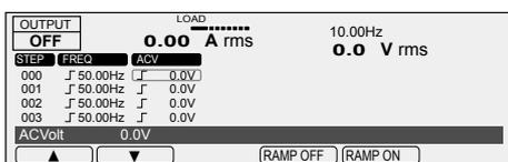
A border is displayed around the ACV item of step 000. Use the rotary knob to specify 5.0 V.
