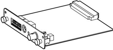
Insert the board in SLOT 3 on the rear panel.
