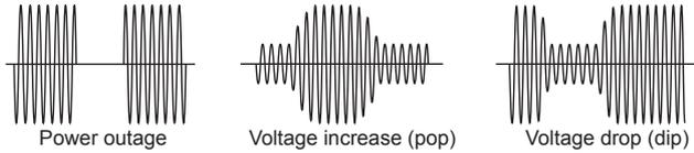
A sine wave is generated during the power line abnormality simulations. Even if you have set a special waveform, a sine wave will be generated as soon as you execute the power line abnormality simulation.
