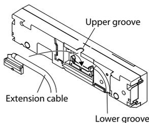
**6** Slide the connector cover back onto the control panel.
