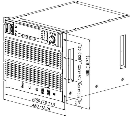
When mounting on a millimeter rack (bracket model KRB400-PCR-LE)
