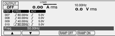
In step 11, the frequency changes from 80 Hz to 40 Hz over 100 ms. Set the frequency of step 11 to 40 Hz, and set the ramp setting to on. This completes the frequency settings.
