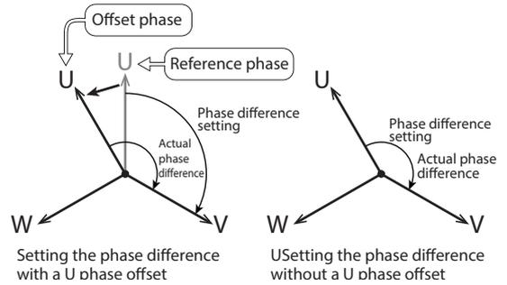
To avoid confusion, we recommend that you turn off the U phase offset when you use the phase sweep feature. For details, see "Phase setting for multi-phase output" in the sequence tutorial of the appendix.
