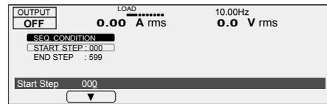
The default starting step number is 0. If START STEP is not 000, use the rotary knob to set it to 000.
