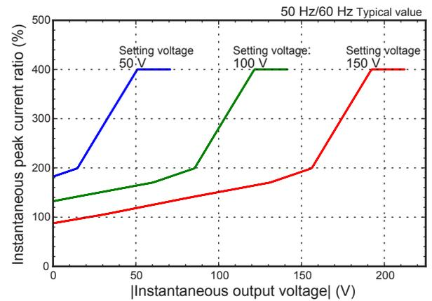
■ Fig.6 Instantaneous output voltage versus instantaneous peak current ratio (AC mode H range, excluding three-phase three-wire output)
