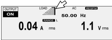
During single-phase, three-wire output (optional), the load level meter displays the U phase at the top and then the V phase.
