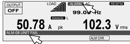
If multiple alarms occur, only the first alarm will be displayed. To display the other alarms that are occurring, press ALM CHK (F5), and then turn the rotary knob.
