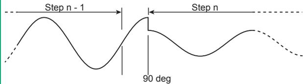
First, set the ending phase angle of the step immediately before the sudden phase change to 90 deg. If the sudden phase change is set to off, the sequence moves to the next step when the phase angle reaches 90 deg after the step time of the previous step elapses, as shown below.
