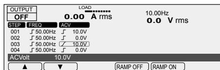
In step 4, the voltage changes from 10.0 V to 0.0 V over 100 ms. Set the voltage of step 4 to 0 V, and set the ramp setting to ON.
