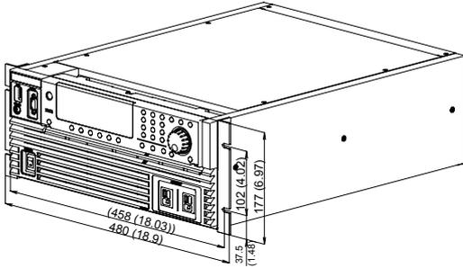
When mounting on a millimeter rack (bracket model KRB200)
