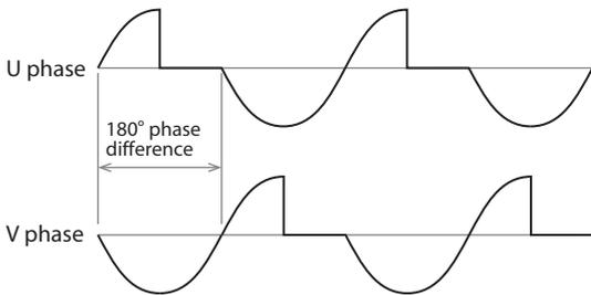
If you want to use two-phase such as in a V wiring connection, set 2P Mode to ON.
