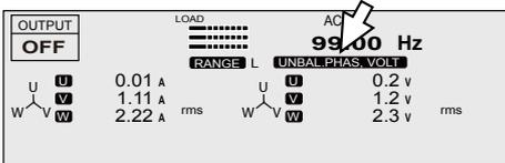
Only one phase can be displayed. Select the phase that you want to display using the PHASE (SHIFT+F) key.
