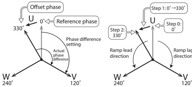
Specify the phase to sweep the U phase with the U phase offset.
