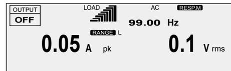
The screen that is displayed that you turn the POWER switch on is called the "home position" (the basic screen). The home position is the top level in the menu hierarchy. All functions are arranged within the menu hierarchy.
