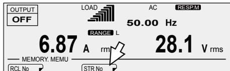
**3 Use the numeric keypad or the rotary knob to select the memory number where you want to store the configuration.**
