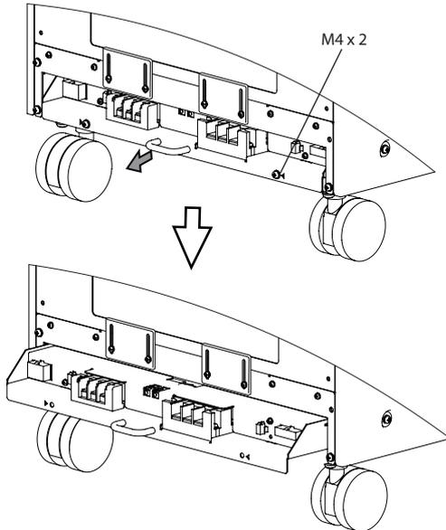
**4** Pull out the stopper to lock the terminal block tray in place.
