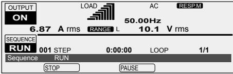
A sequence is complete when all steps are complete. The condition that the PCR-LE Series is in when a sequence is completed is the condition specified in the last step of the sequence.
