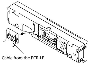
**4** Connect the cable from the PCR-LE Series to the control panel extension cable. Use the band and the bracket to fix the control panel extension cable to the PCR-LE Series.
