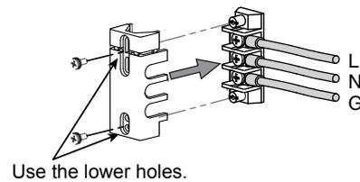
Twist the load wires (L and N), and connect between the output terminal and load with the shortest wires possible. If you cannot twist the wires, we recommend that you run the wires alongside each other and tie them together at several points with cable ties.
