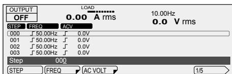
You can edit the step that has a border around its item or value. 000 is selected. If 000 is not selected, use the rotary knob to select it. You can also select steps by pressing STEP (F1) and then using the rotary knob.
