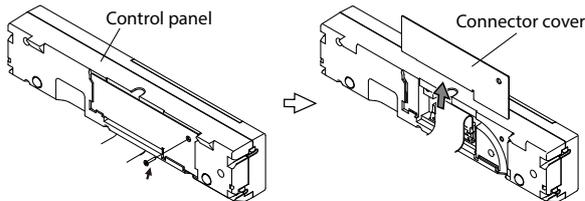
**3** Remove the cable that is connected to the control panel.
