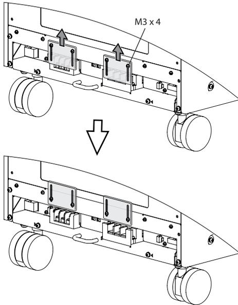
**3** Remove the two terminal block tray screws, and then pull the tray out.
