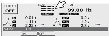
The full scale bar (the right-most bar that lights red) of the load level meter lights on the verge of an overload.
