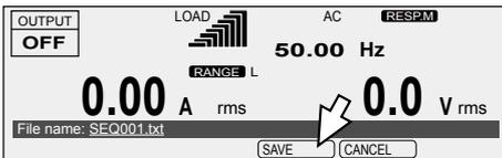
Press SAVE (F4) to save the settings. Do not remove the USB memory device until "File was saved" disappears.
