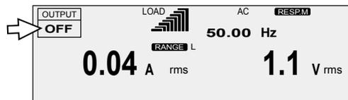
If a protection function is activated and the product is in the alarm state, the output is turned off.
