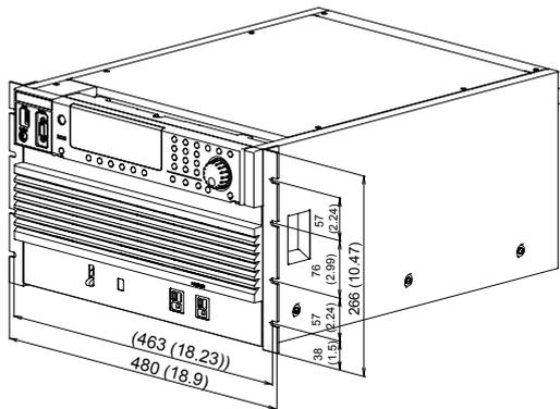
When mounting on a millimeter rack (bracket model KRB300)
