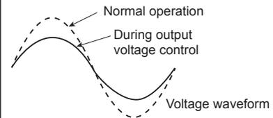
\*1. This is calculated as an rms value. The current limit may be exceeded for a few seconds because of the relationship between the measurement processing time and the voltage resolution. The current may oscillate (increase and decrease) while it is being controlled.
