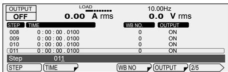
Press TIME (F2) to set the step execution time. Press  $\blacktriangle$  repeatedly until you reach the time setting of step 000. Press 100US (F6), use the numeric keys to enter 100 (0:00:00.1000), and press ENT. The microsecond resolution is 100  $\mu$ s.
