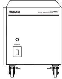
By using the control software (SD009-PCR-LE), the dip simulator (DSI1020/ DSI3020), and the PCF-LE Series, you can perform voltage dip, short interruptions, and voltage variation immunity tests in accordance with IEC61000-4-11 (2004).
