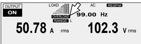
Press I and then TRIP (F2) to select the action to perform when the limit is exceeded.
