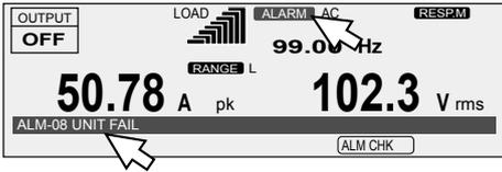
During master-slave parallel operation(optional), if an alarm occurs on one unit, the entire system's output will be turned off.
