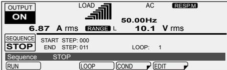
If you want the output to turn off when the sequence is complete, you need to add a last step that turns the output off.
