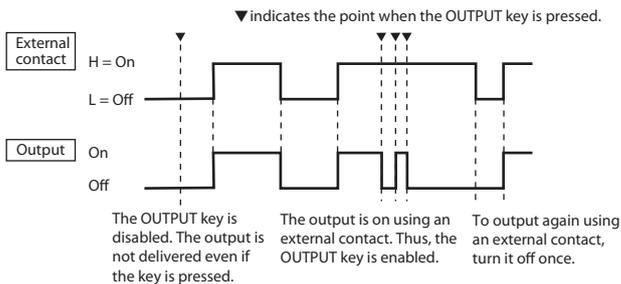
When a sequence is running, the output on/off control through external contacts is invalid.
