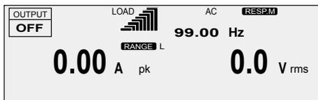
If the POWER switch is turned on for the first time after purchasing the PCR-LE Series, the PCR-LE Series starts up using factory default settings. For all other cases, the PCR-LE starts up using the settings that were in use the last time that the POWER switch was turned off.
