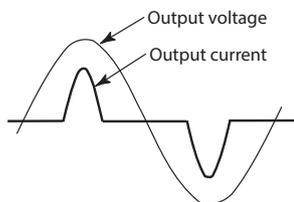
As shown in figs. 10 to 13, keep the maximum peak current near the peak value of the instantaneous output voltage from exceeding four times the rated maximum output current.
