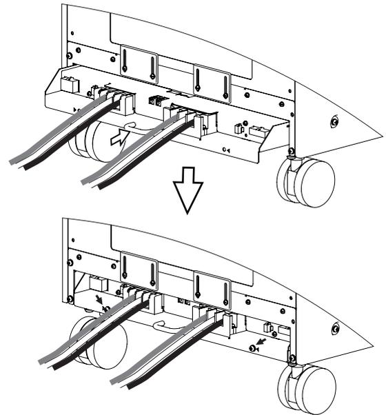
**8** Slide the two terminal box covers down until they are touching the wires, and then use the four screws to fix the terminal box covers in place.
