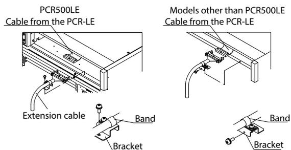
**5** Connect the control panel extension cable to the control panel.
