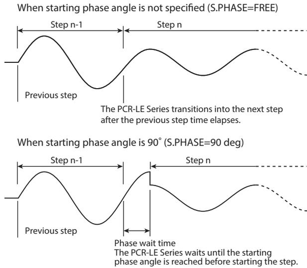
If you set the ending phase angle, the PCR-LE Series will end the step when the specified phase is reached.
