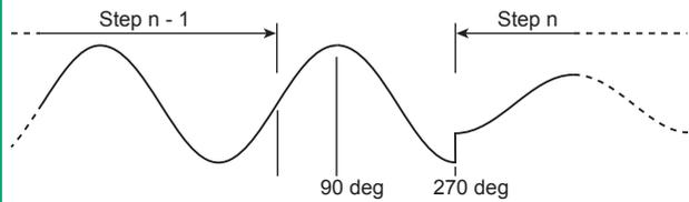
Lastly, set the sudden phase change to on. When the phase angle of the previous step reaches 90 deg, the sequence changes to the next step. The next step begins at 270 deg.
