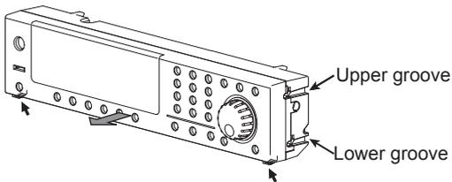
While pressing in the two locations (indicated by this arrow in the figure), detach the panel by pulling it toward you.
