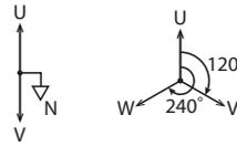
Describes the waveforms that are produced for single-phase, three-wire output and three-phase output.
