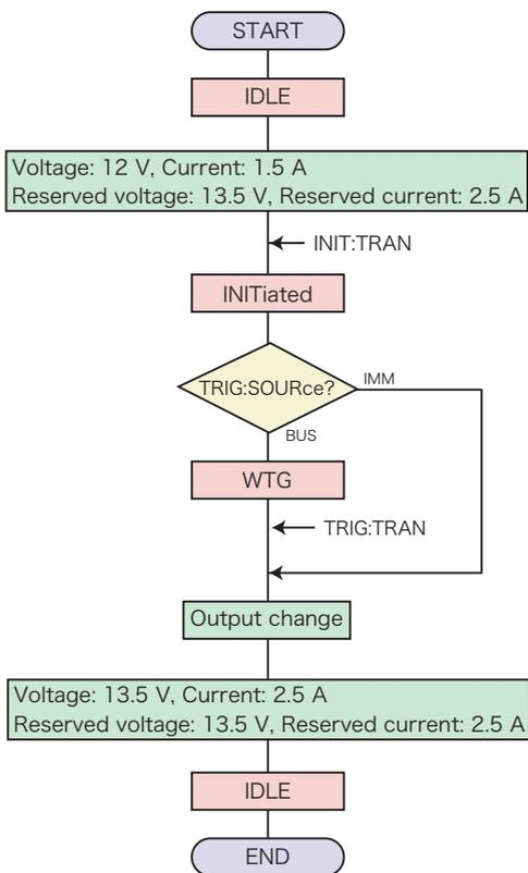
The `TRIGger:TRANSient:SOURce` command sets the trigger source to `BUS`, or `IMMEDIATE`.
