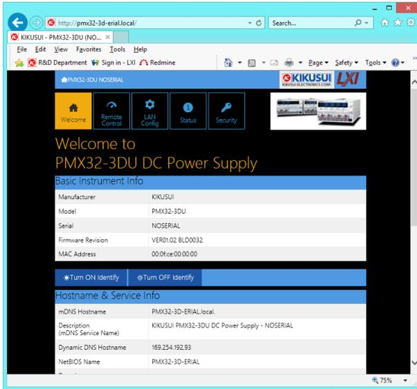
**Turn ON Identify:** The LAN LED on the front panel of the connected PMX blinks so that you can identify it.
