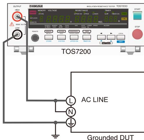
Insulation resistance test across the AC LINE and chassis of the DUT
