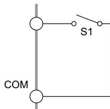
Use a make contact such as a relay or switch to set the input terminal to the Low level.
