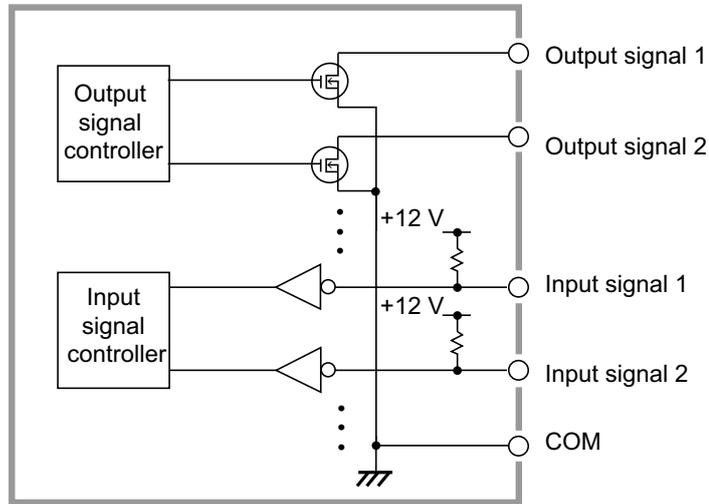
Internal Configuration of the SIGNAL I/O Connector
