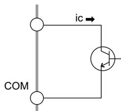
Use a logic element such as a transistor in place of a switch in the above example. Consideration should be given to pulling up the transistor's collector current,  $i_c$ , by 5 mA or more.
