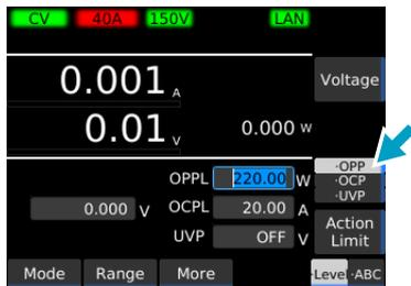
**3 Use the numeric keypad or the rotary knob to enter the power value.**
