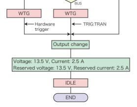
The TRIGger:TRANSient:SOURce command sets the trigger source to BUS, TRI-GIN, or IMMediate.
