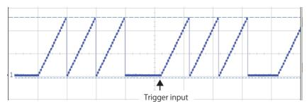
In a step with voltage transition set to RAMP, the voltage changes linearly (actually, step transition at 100 ms intervals) from the voltage setting of the previous step to the specified voltage.
