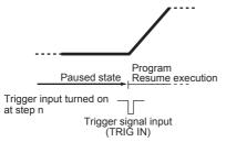
When trigger input in the next step (n+1) is set to on, if a trigger input is received while step n is executed, the step immediately switches to step n+1.
