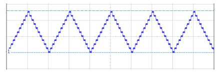
In a step with voltage transition set to RAMP, the voltage changes linearly (actually, step transition at 100 ms intervals) from the voltage setting of the previous step to the specified voltage.
