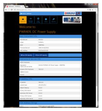
Turn ON Identify: The LAN LED on the front panel of the connected PWR-01 blinks so that you can identify it.
