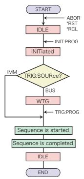
To start a sequence immediately, set the trigger source to IMMediate, and then use the INITiate:PROGram command.
