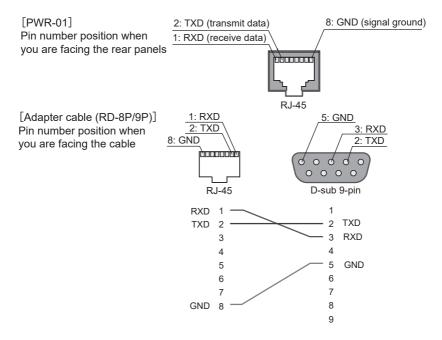
TRIG-IN is assigned to pin 7 of the this product's RS232C connector. TRIG-IN is used for synchronized operation.
